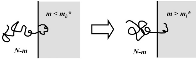
FIGURE 4 A hairpin entry with m_l^* < m < m_h^* and only one tail in the deep region leads to a linear translocation. The chain enters the shallow region as a hairpin but m does not exceed the hairpin critical insertion size m_h^* . The chain end forming the hairpin has no entropic penalty to prevent itself from proceeding into the shallow region and gaining electrostatic energy. If m is larger than the linear critical insertion length m_l^* , linear translocation occurs.
